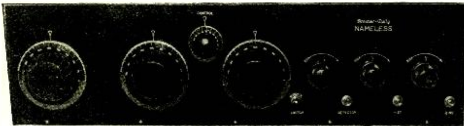
Front view of the "Nameless" set, which in many respects resembles the conventional neutrodyne, save for the small compensating condenser as seen between the second and third dial.
