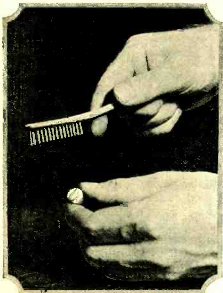
Fig. 10.—Using tooth brush and alcohol to clean surface of detector crystal.
